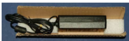
Fig. 7 Place power adapter with its cord on the side of with the larger piece of foam in cardboard encasing.
